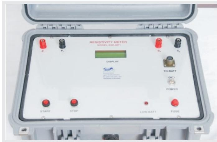
The IGIS Microprocessor based Signal Enhancement Resistivity Meter Model SSR-MP1 is a high quality microprocessor based data acquisition system incorporating several innovative features. The instrument design incorporates several advanced techniques of digital circuitry to make it reliable geophysical tool that provides high quality data useful for all types of mineral and groundwater exploration research etc.
